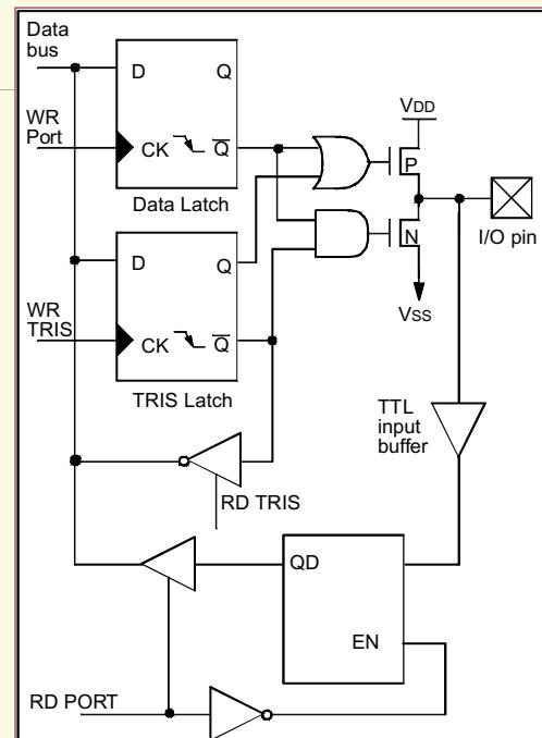
Note: I/O pins have protection diodes to Vdd and Vss.
